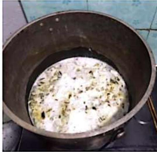
Figure 15. Bleaching husks in 6% NaOCl
