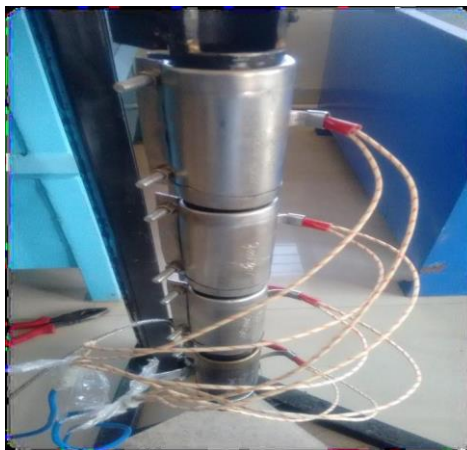
Fig. 4.2 Assembly of Band Heater
