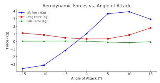
From the above plot, Aerodynamic Forces vs. Angle of Attack: Lift force increases with  $\alpha$ , peaking at 10°, while drag force remains relatively low up to 5°.
