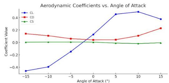
From the above plot, Aerodynamic Coefficients vs. Angle of Attack:  $C_L$  shows a steady increase, while  $C_D$  remains minimal around  $\alpha = 5^{\circ}$  before rising significantly.
