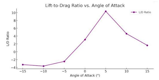
From the above plot, Lift-to-Drag Ratio vs. Angle of Attack: The L/D ratio reaches a maximum value of 10.34 at  $\alpha = 5^{\circ}$ , indicating the most efficient aerodynamic performance.
