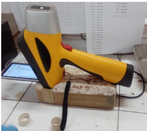
Photo 3: pXRF device used for major oxide determination
