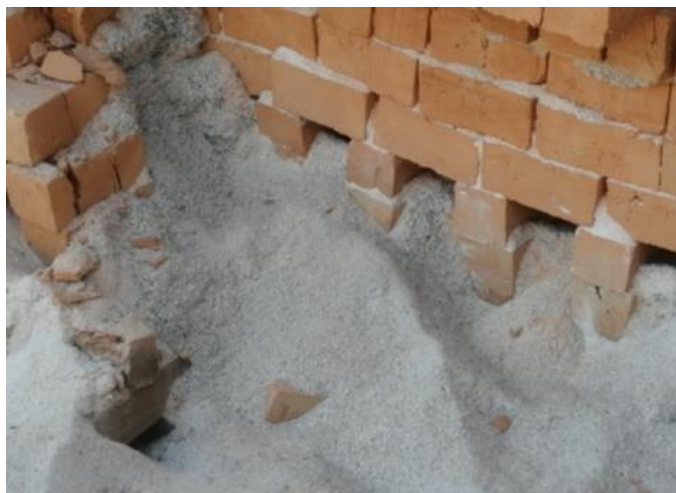
Photo 1: Rice husk ash “Maika” in an artisanal brick kiln.
