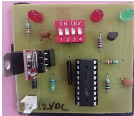
Fig 1. Transmitter section placed at the poles
