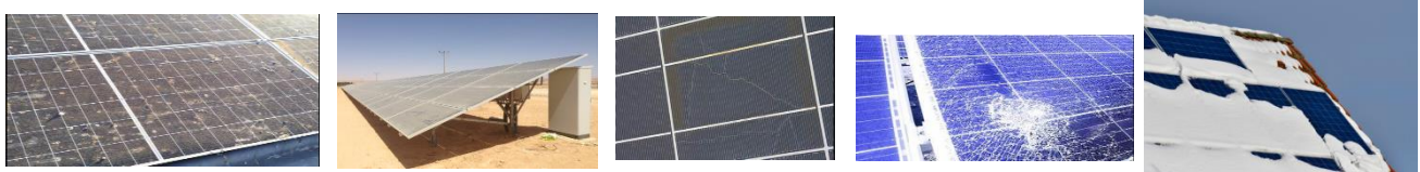
Fig 1: a) Bird Dropping; b) Dusty; c) Electrical Damage; d) Physical Damage; e) Snow Covered
