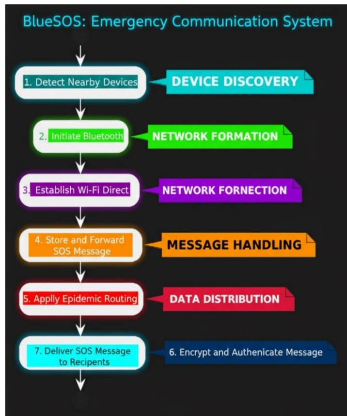
Fig 1. Bluesos: Offline SOS System Using Epidemic Routing Algorithm Workflow
