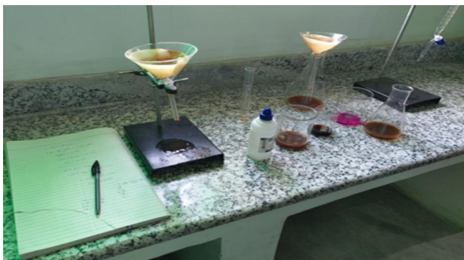
Fig.3: Titration of Kombucha Sample for alcohol percentage estimation
