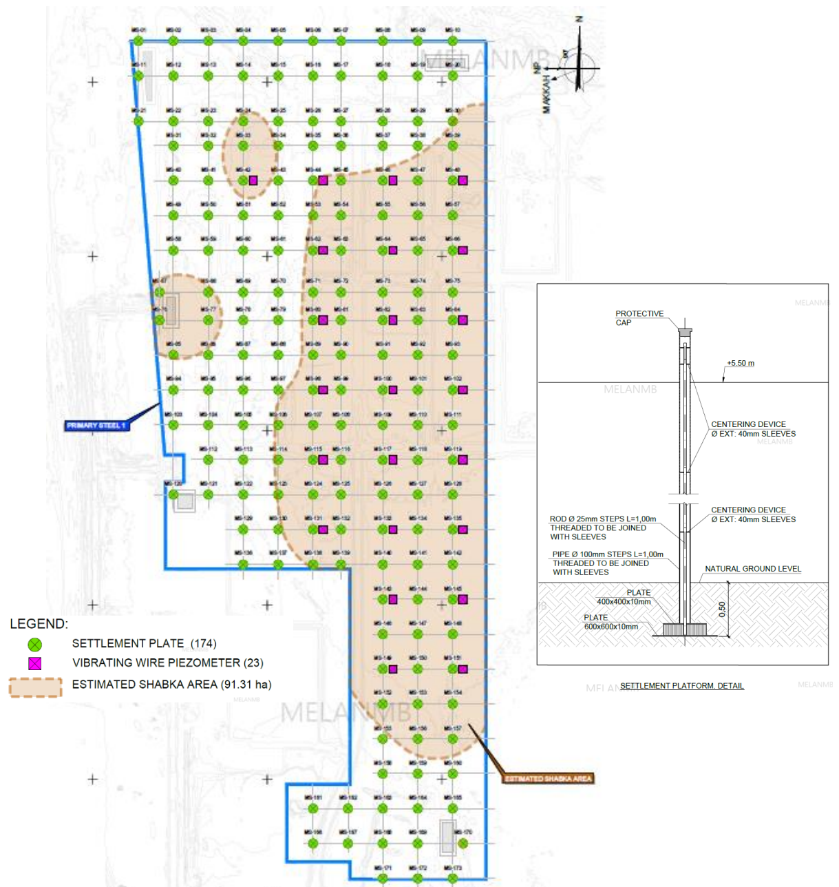
Figure 6.0: Settlement marker layout and detail
