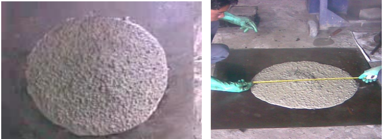
Fig. 1 - (a) Slump Flow; (b) Flow Measuring.
