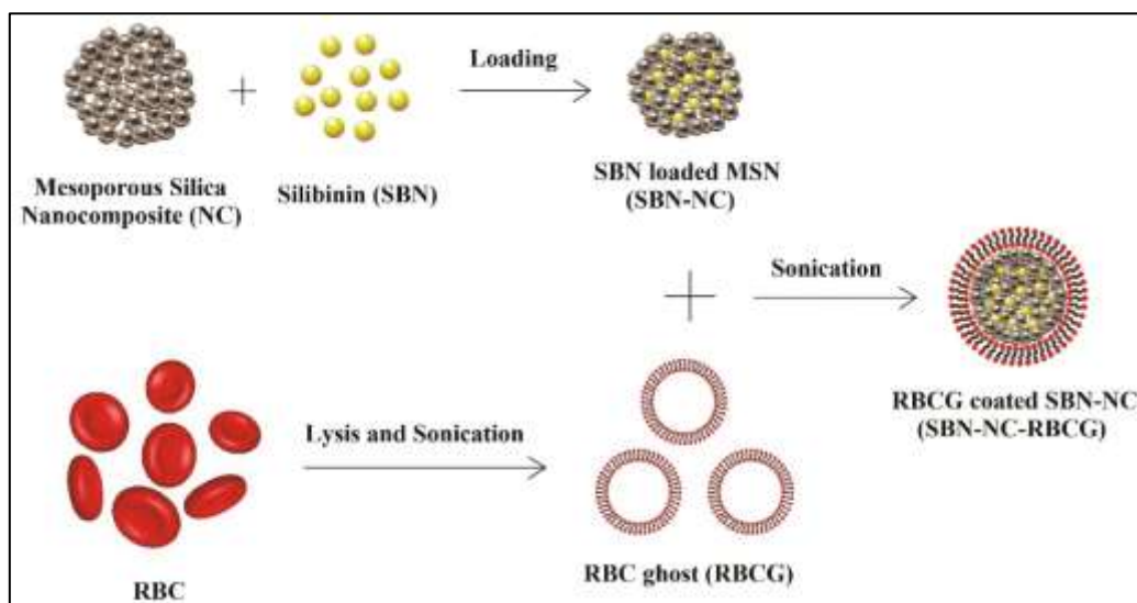
Fig. 10 : Method preparation of coating of RBC-ghost on the surface of SBN loaded NC [40]
