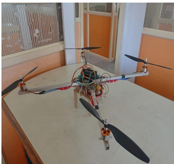
Plate1. Complete assembly view of drone sprayer
