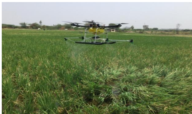
Plate3.Field Efficiency assessment of the drone-mounted Liquid dispenser in Rice and ragi crop
