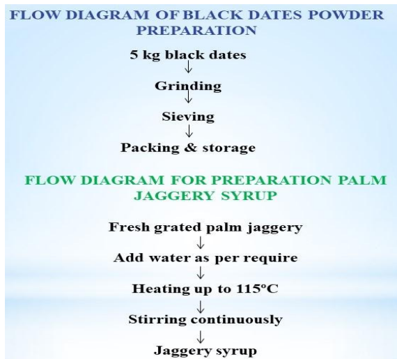
Figure-3: Flow diagram of black date powder and palm jaggery syrup
