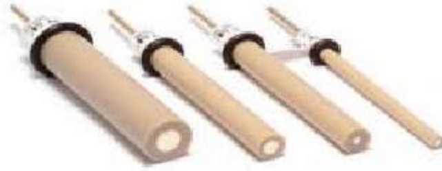
Fig 1.0: Metal encapsulated in epoxy resin serves as working electrodes (Sumayah, 2019).
