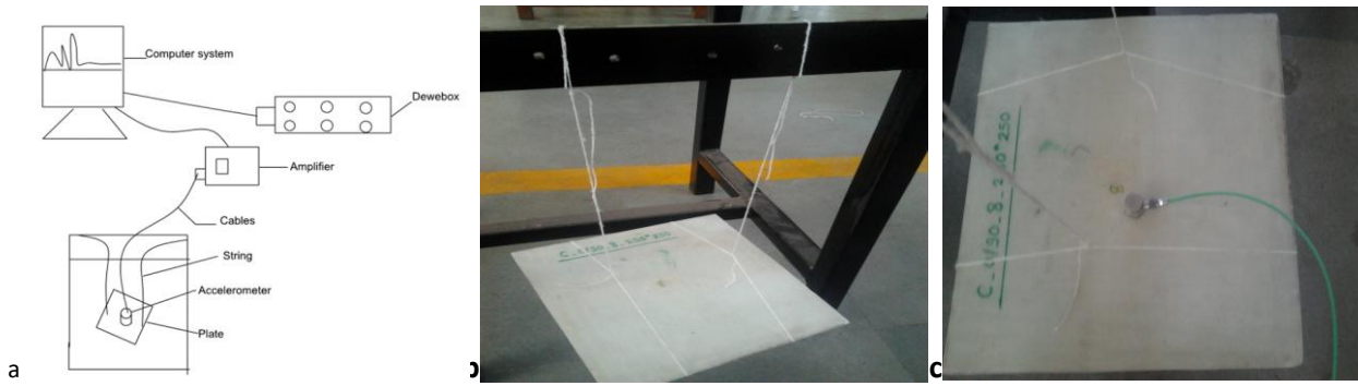
Fig 2–(a)Schematic of Experimental Setup; (b) Plate setup; (c)Accelerometer mounting
