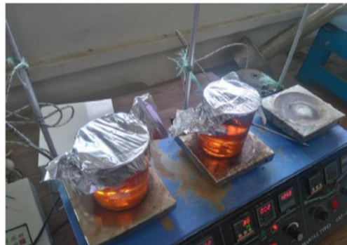
Figure 3.2 Preparation of Blends using the magnetic stirrer
