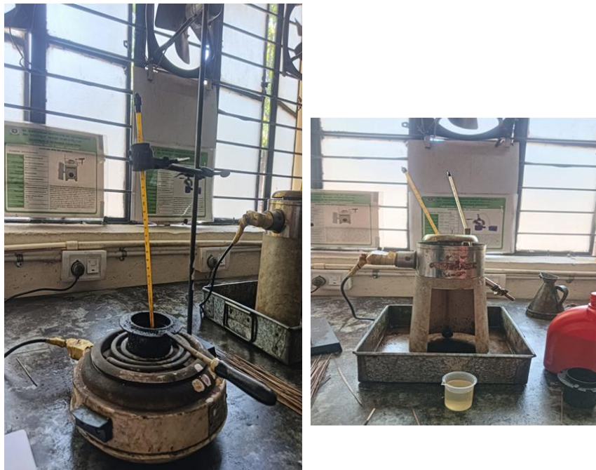
Figure 8: Cleveland open cup apparatus
