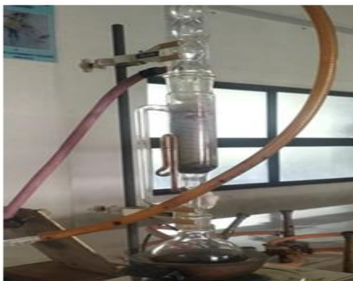
fig: The extraction of samples using the Soxhlet method
