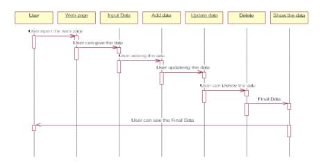
According to UML's Unified Modeling Language standards, a sequence diagram works as an interaction diagram that specifies the interactions between the processes as well as the order in which said interactions occur. Its a subclass of Message Sequence Chart. This diagram shows the objects and classes involved in a particular scenario and depicts the order of messages passing between the objects or classes to counter the defined tasks and process.
