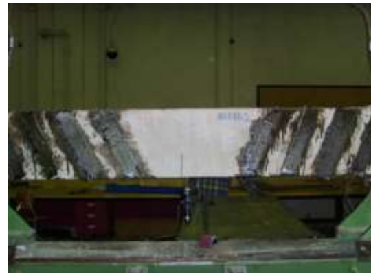
Fig.1.8: Inclined strip system
