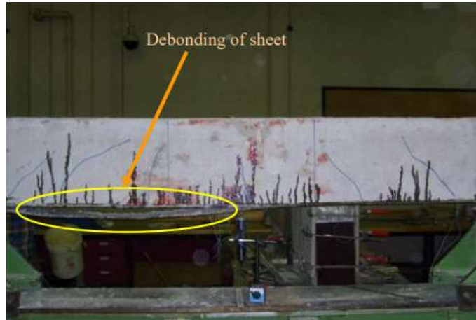
Fig.1.5: Debonding of sheet failure
