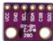
Figure 4. Measure Temperature, Pressure and Altitude (BMP280).
