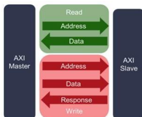
Figure 1: AXI read and write channel
