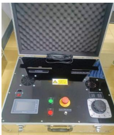
Figure 2 Herbal extract machine using combined energy of pulsed electric field and ultrasonic. Mobile, low cost
