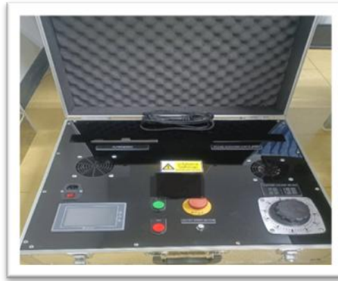
Figure 1 Low-cost mobile combined electric pulse field and ultrasonic herbal extractor.
