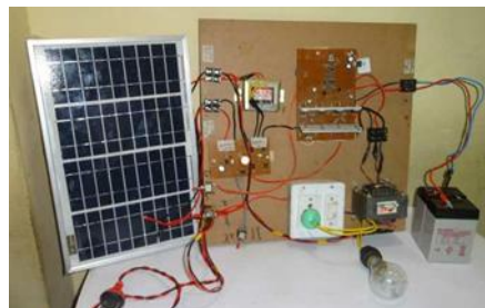
Fig 3 Smart Solar Inverter with IoT Working Model
