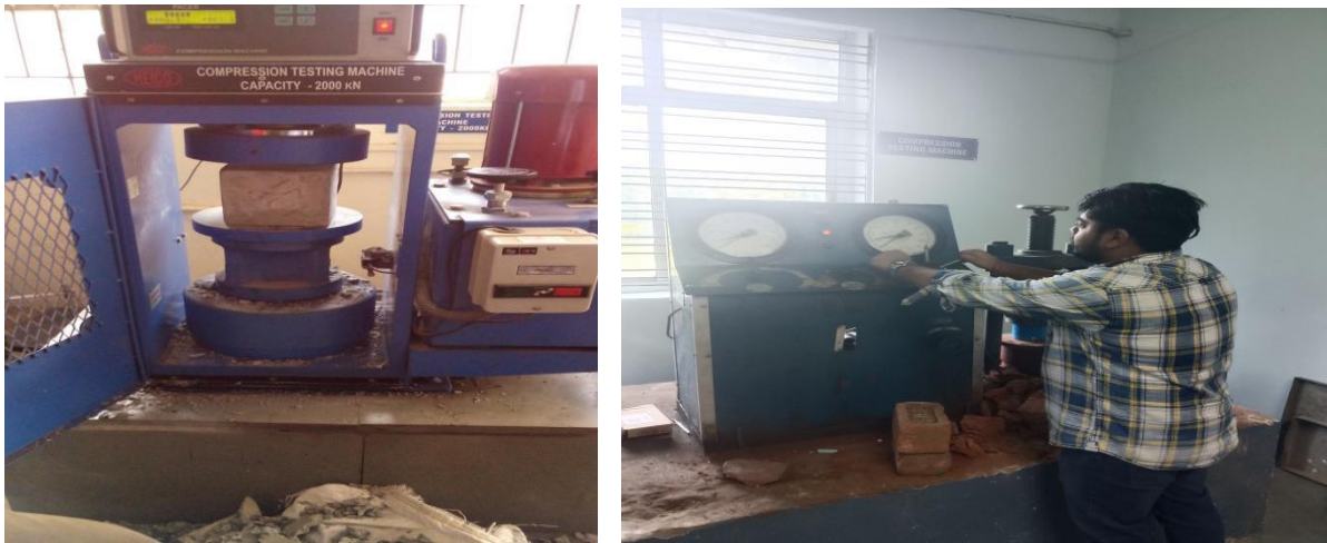
Figure 2 Compression Testing Machine used in present investigation Testing of Cubes
