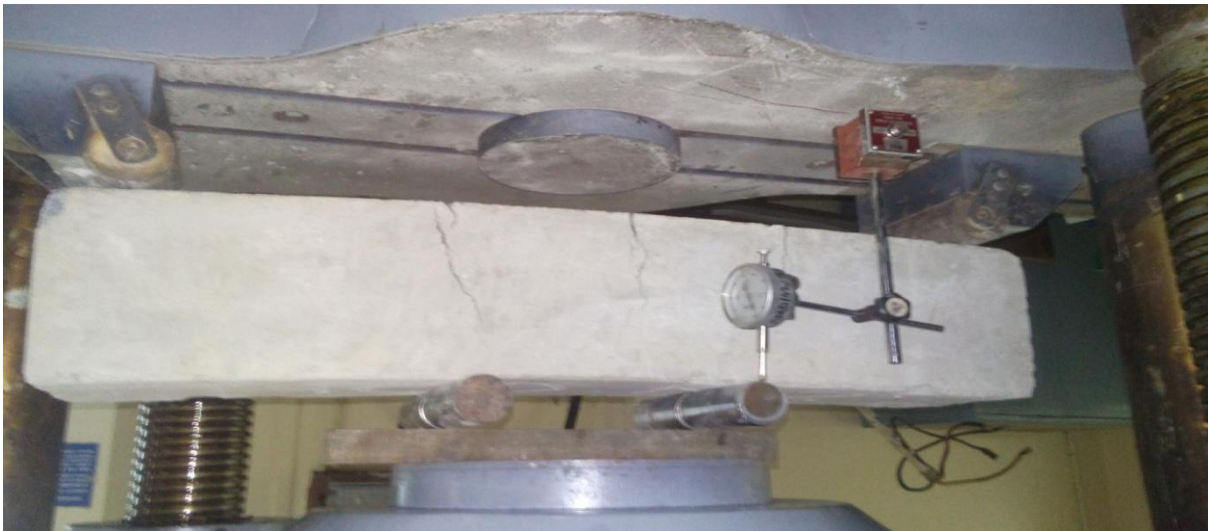
Figure 3 Compression Testing Machine used in present investigation Testing Of Beams
