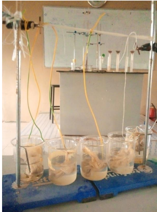
Fig.1. test for water absorption
