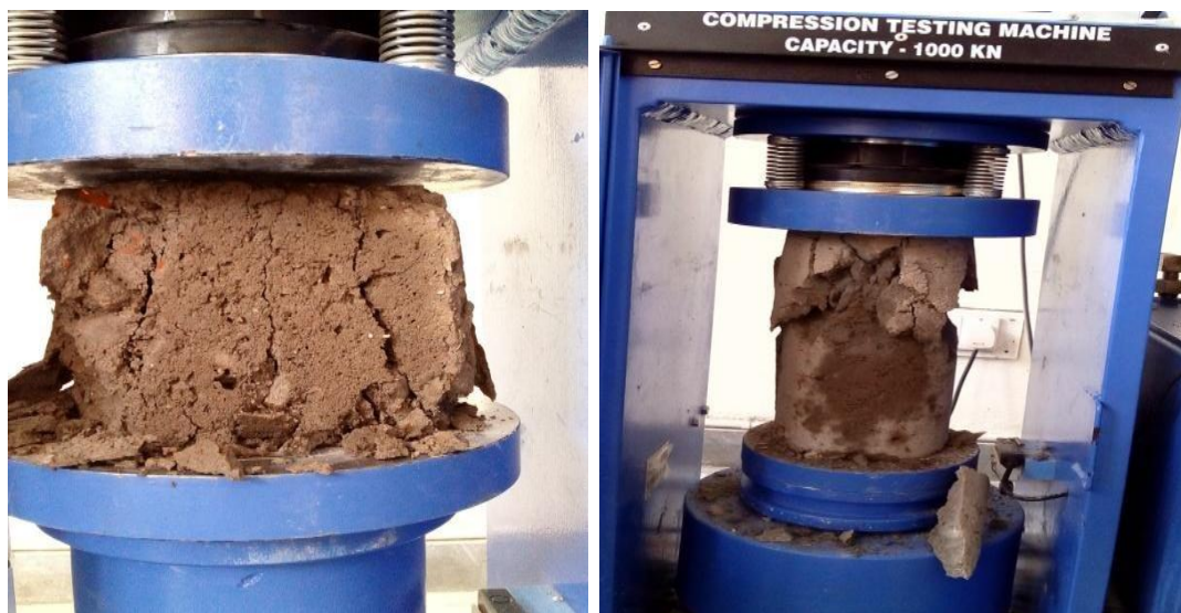
Figure 6: Cube and Cylinder testing
