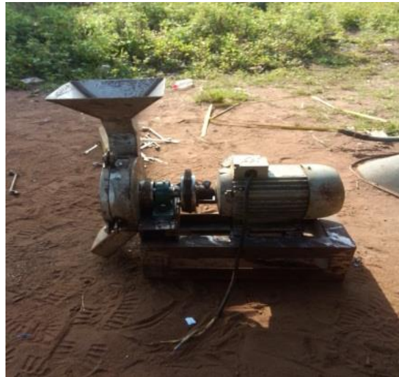
Fig 3: Fabricated hammer mill
