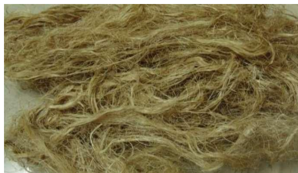
Fig. 4.1 Chemically treated fiber.
