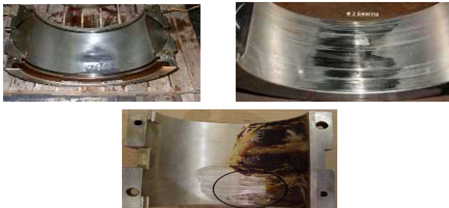
Fig. Failure modes of hydrodynamic bearing
