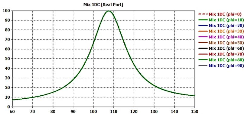
Figure 6: Incident Angle Plot for the Implemented Absorber
