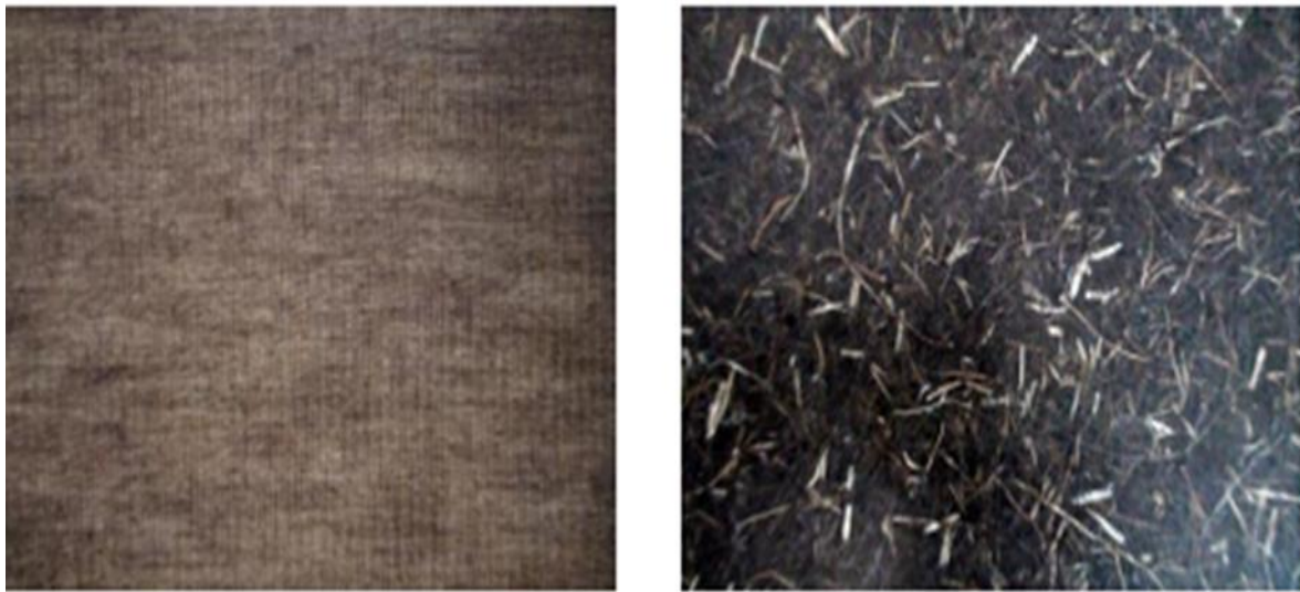
Fig. 4 - Flax fiber unidirectional and non-woven fiber after dry Mold
