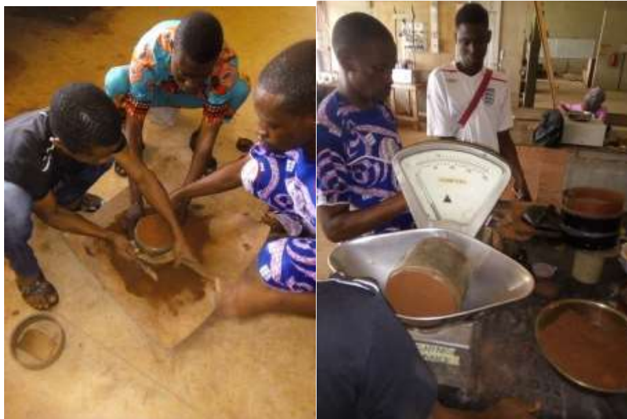
Fig 3: Compaction Test in progress
