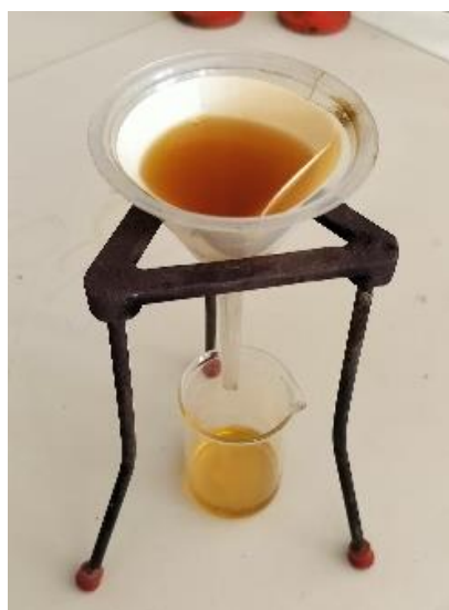
Figure 13. Filtration of bael extract
