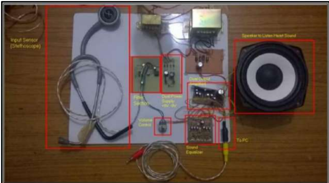
Figure 5.2 Hardware Design for Integrated Electronic Stethoscope
