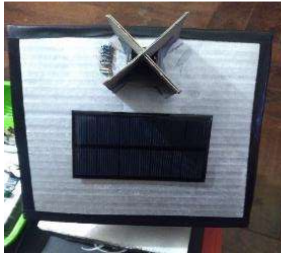
Fig. 16 Panel Bracket showing sensors
