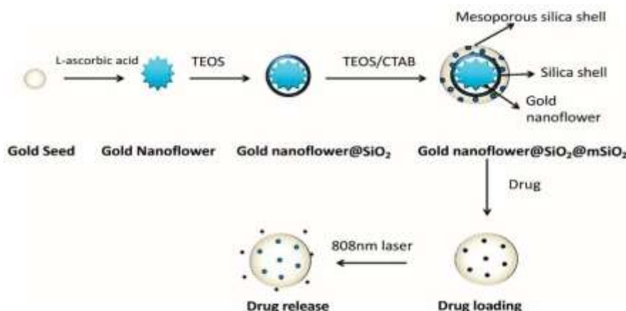
Fig No 5: Schematic representation of the synthesis of gold nanoflowers for oral cancer treatment. [109].
