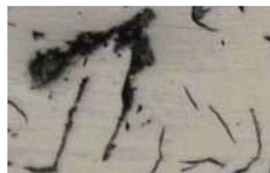
Fig. 2 Micrograph of flakes in Grey Cast iron.
