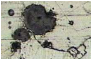
Fig.1 Micrograph of spheroid In ductile iron.
