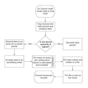
Algorithm 1: Algorithm for data compression in Fog node Input: Generic Numerical Sensor Data Output: Compressed Numerical data
