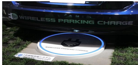
FIG NO 4: Wireless battery charging
