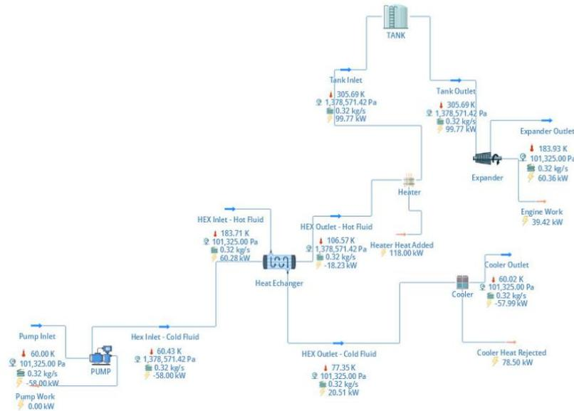
Fig. R1. Organic Rankine System Using Nitrogen (Air)
