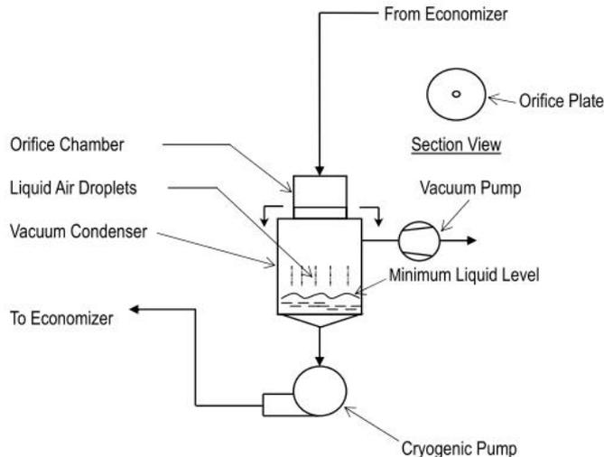
**Figure 2-5.** Air Passing through Nozzle (Orifice) and Expanding in a Vacuum Condenser to Form Liquid Air Droplets
