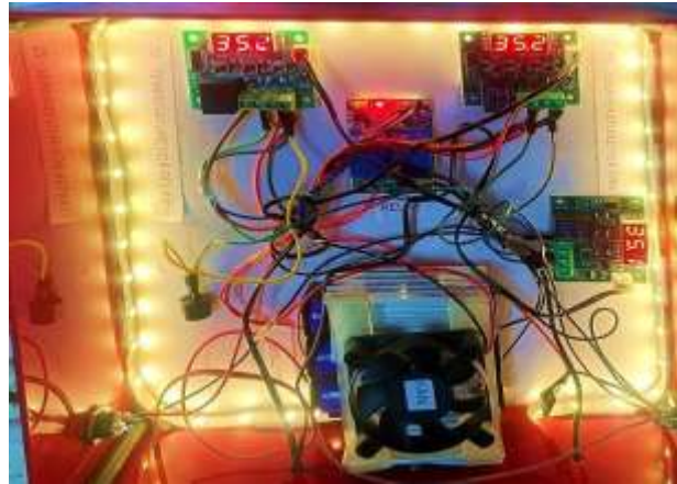
Figure 1: Prototype image of Thermal Safety System for Electric Vehicles.
