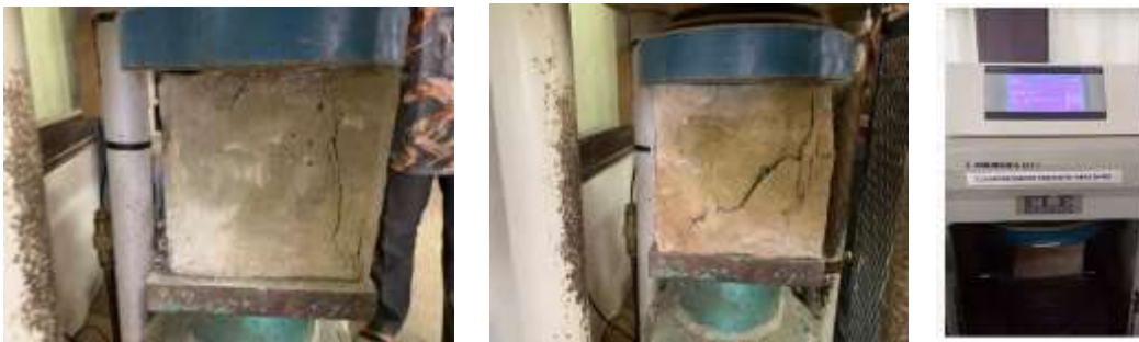
Figure 3: Testing the compressive strength of concrete
