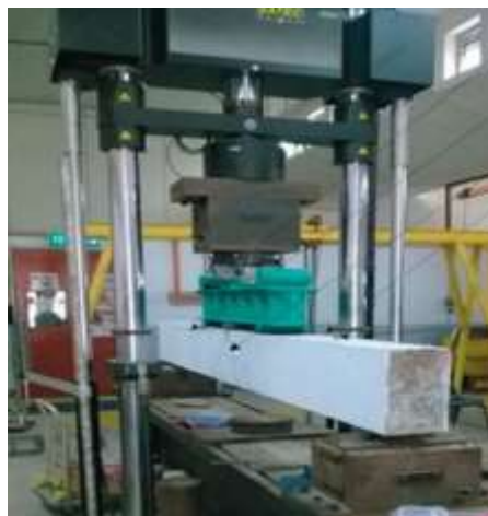
Fig. 4 - Beam test setup for experimental investigation
