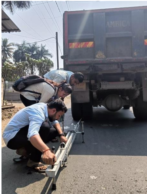
Insert Instrument Between Dual Wheels of Truck
