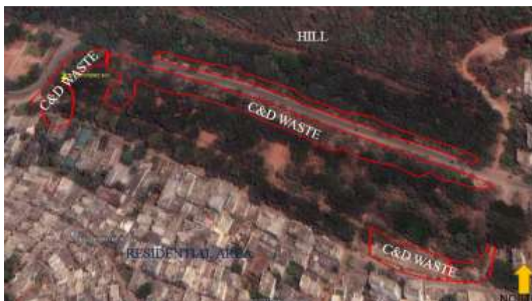
Fig. 4: Satellite image showing C&D waste scattered over 4.5 acres of open land in the study area.
