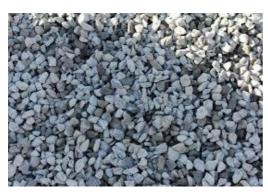
The coarse aggregate used in this study consisted of 20 mm and 10 mm downsize locally available crushed stone obtained from nearby quarries. Physical properties were determined as per IS: 2386-1963 standards, revealing a specific gravity of 2.68 and water absorption of 0.25%.
