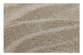
Neighborhood clean waterway sand of Zone II, conforming to IS 383-1970 standards, was employed as the fine aggregate. The sand underwent sieving with a 4.75 mm sieve to ensure it was free from clay, silt, and organic impurities. Physical tests were conducted to assess its gradation, fineness modulus, specific gravity, and bulk modulus in accordance with IS: 2386-1963.
