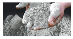
For this study, ordinary Portland cement of 43-grade conforming to IS 12269-1987 was utilized. The cement underwent thorough checks for freshness and consistency, ensuring it was devoid of any lumps and maintained its purity.
