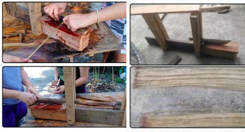
Figure 2: Decortication of fiber using D-I-Y decorticator made out of wood and knife.
